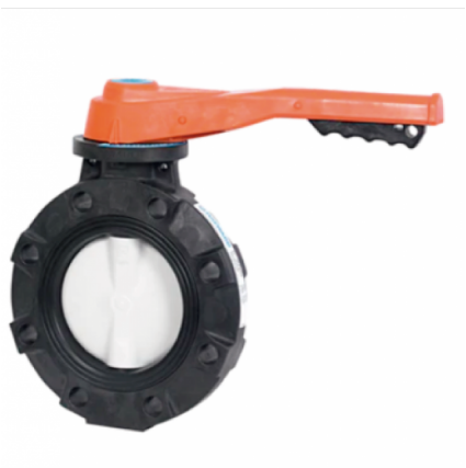
BYV SERIES GFPP 2" BUTTERFLY VALVE, w/EPDM, Handle Lever
